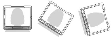
Place the TD Pilot on your mounting system or a stable surface in front of the user at, or slightly below, their eye level. If their head is tilted left or right, tilt the TD Pilot to match. It is important that the angle of the screen surface match the angle of the user's face. Most users, when seated at a table or desk, will need to have the TD Pilot positioned higher than the table surface.
