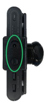
Ensure the Powerbank is properly in place, and the cradle edges are securely surrounding the Powerbank.
