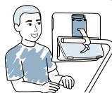
Optimised positioning for both the device and the individual is necessary for successful use. Place the device on the mounting system or on a table using the Adjustable Base, in front of the user. If you are using Gaze Interaction, review Tips for Eye Tracking.
