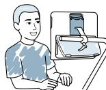
Optimized positioning for both the device and the individual is necessary for successful use. Place the device on the mounting system or on a table using the Adjustable Base, in front of the user. If you are using Gaze Interaction, review Tips for Eye Tracking.
