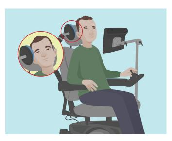
If a switch is not worn on the body, switches can be positioned with a mounting plate and mounting arm. Mounting accessories are available through Tobii Dynavox.
