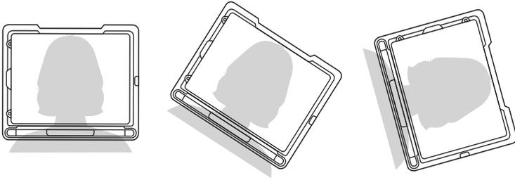
Place the TD Pilot on your mounting system or a stable surface in front of the user at, or slightly below, their eye level. If their head is tilted left or right, tilt the TD Pilot to match. It is important that the angle of the screen surface match the angle of the user's face. Most users, when seated at a table or desk, will need to have the TD Pilot positioned higher than the table surface.
