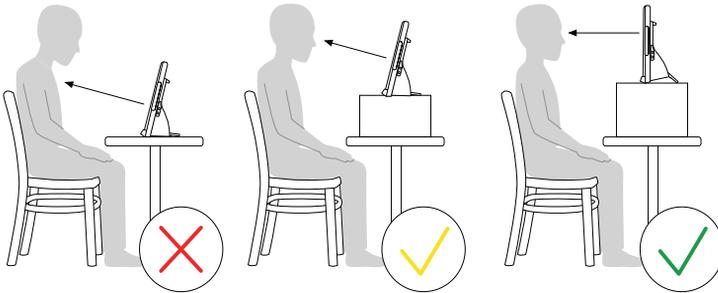
You may need to refine the position of the device during the Calibrate steps on the next page. Always adjust the position of the device to suit the user, not the other way around.
