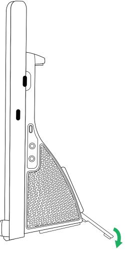
Adjust the angle of the Adjustable Stand to give the TD Pilot a good alignment with the user.
